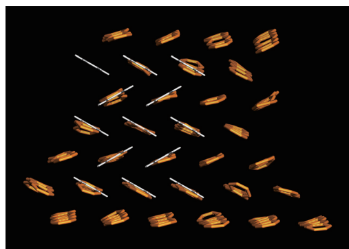
Fig. 10 Comparison of the structures found in Figs. 8-9 (orange) and an experimentally formed crystal structure of pentacene (white). Both have herringbone structures.
